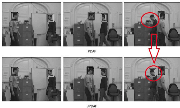
Fig. 3. In a study of Probabilistic Data Association Methods documented by Rasmussen and Hager (2001), there was an illustration of tracking results across homogeneous regions for PDAF and JPDAF methods. Clearly, the PDAF model fails to maintain the track once the object has been occluded for a short period of time, indicating an issue with re-identification.
