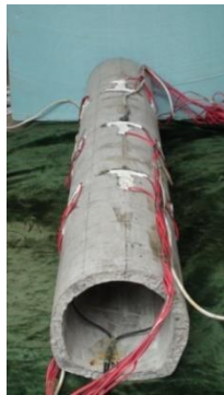
Fig. 2 Horseshoe shape tunnel model
