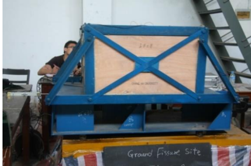
Fig. 1 Shake table tunnel model setup
