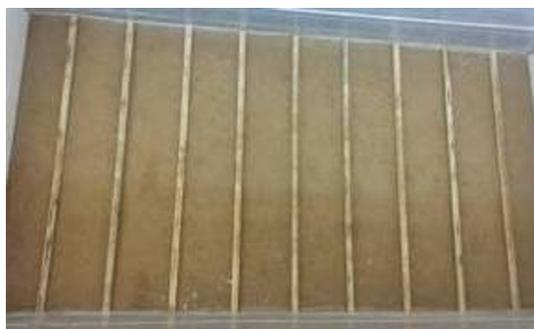
Fig. 7. Treatment of friction at the box bottom.
