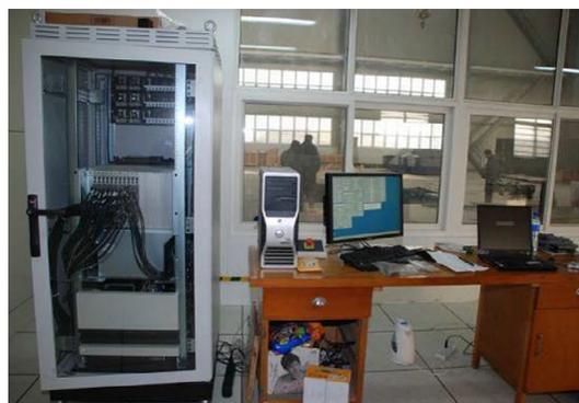
Fig. 5. Shaking table control system.
